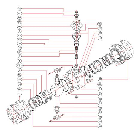
Note: body cover bolt (152) only for DN150(DN200 RB) PN10-40 and DN100(DN150 RB) PN63-100
